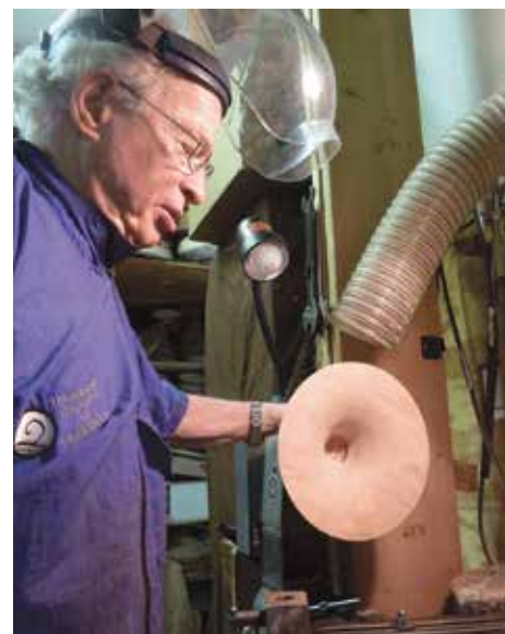
Phil with a trademark trumpet form on his Delta Homecraft lathe. Five-inch risers and a custom toolrest give this machine exceptional capacity for its mass.
